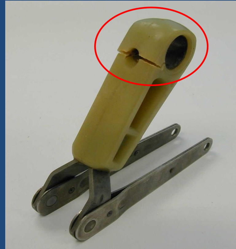
Faulty high voltage insulating operating arm
