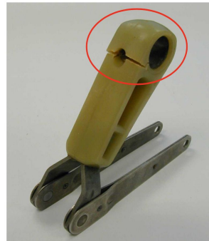
Faulty high voltage insulating operating arm
