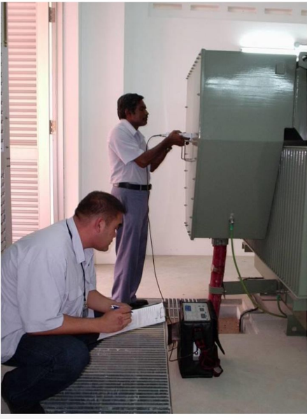
TEV Partial Discharge detection
