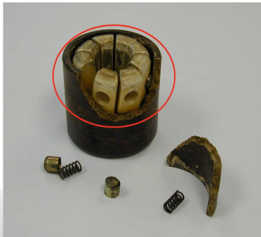
Faulty tulip contact assembly
