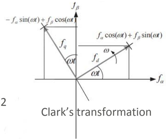
$$\begin{bmatrix} f_\alpha \\ f_\beta \end{bmatrix} = \sqrt{\frac{2}{3}} \begin{bmatrix} 1 & -\frac{1}{2} & -\frac{1}{2} \\ 0 & \frac{\sqrt{3}}{2} & -\frac{\sqrt{3}}{2} \end{bmatrix} \begin{bmatrix} f_u \\ f_v \\ f_w \end{bmatrix} \quad \text{Equation 1}$$
