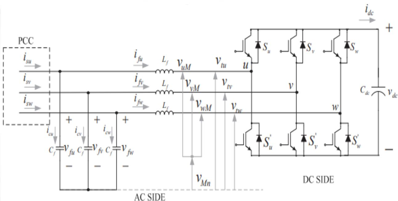
The series active power filter is structured as a voltage source inverter circuit, uses IGBT as a power electronic switch.
