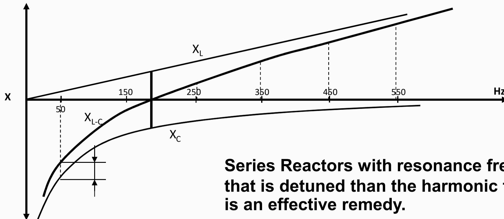
Series Reactors with resonance frequency that is detuned than the harmonic frequency is an effective remedy.
