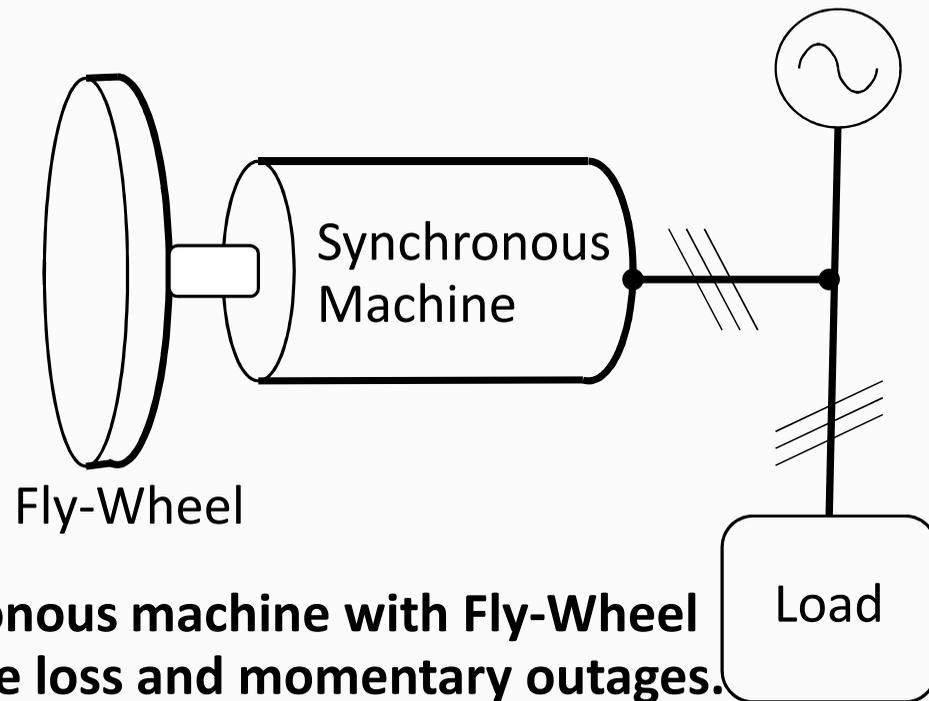
Synchronous machine with Fly-Wheel
