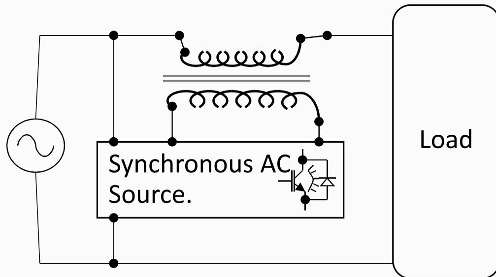
Series Boost Buck Converter Schematic
