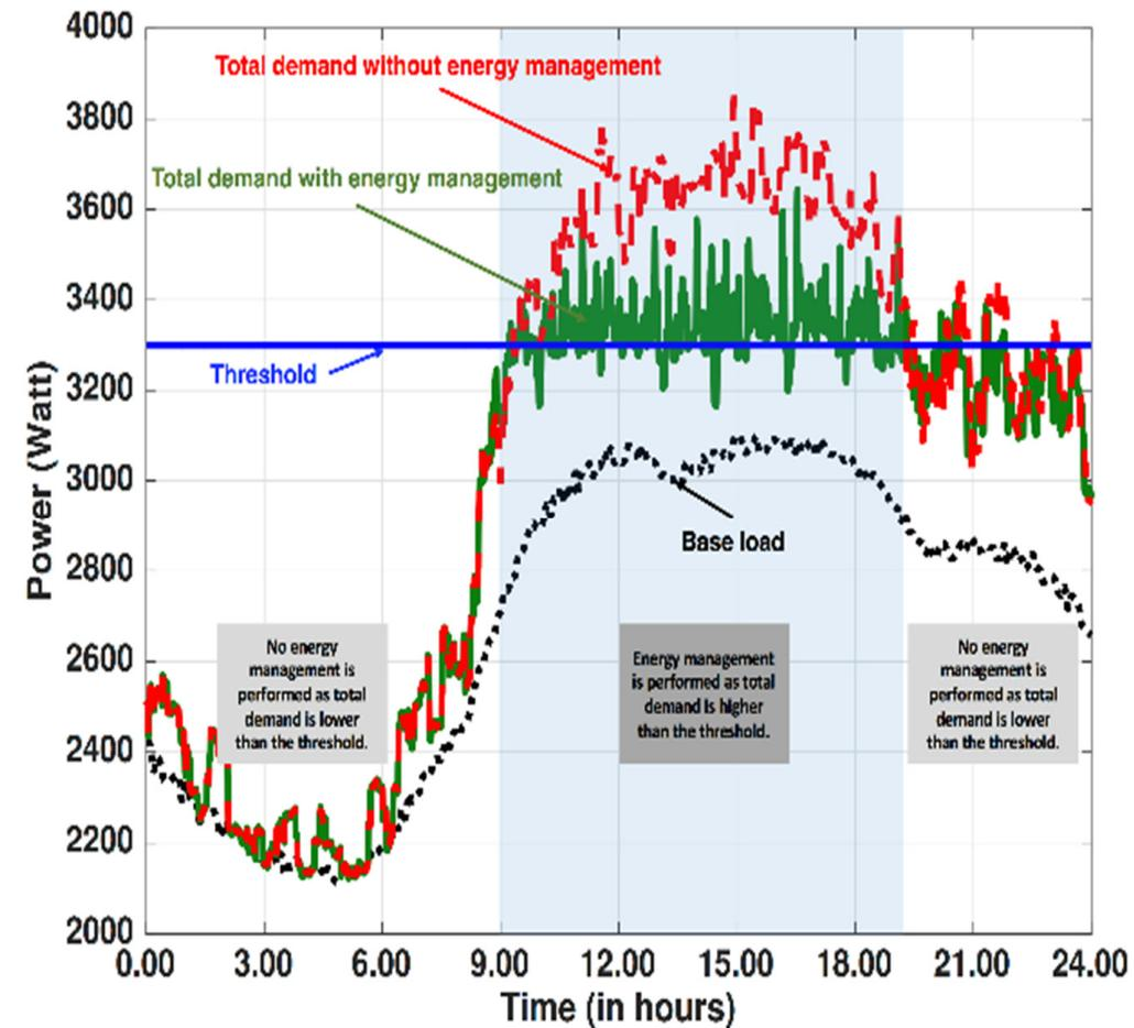
Control mechanism that are suitable for managing energy demand through smart plugs, which is capable of keeping the peak load within a range that was 14.28% lower than the original peak load during the experiment period for the considered scenario (Published in *IEEE Access*, 2015).
