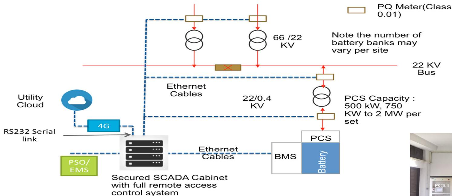
Installed at Bedok 22 KV at one of the outgoing feeder (1 MW/3 MWh)
